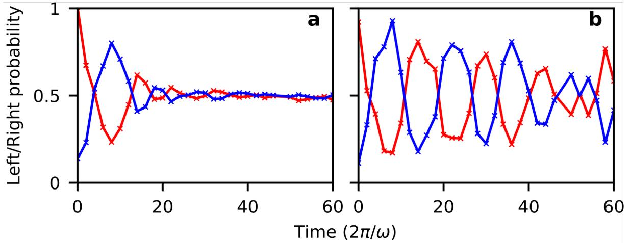
**Fig. S9. Damping of oscillations with the number of atoms.** Comparison of the chaos-assisted tunneling oscillations for two different atom numbers: **a**  $N = 1.2 \pm 0.2 \times 10^5$  and **b**  $N = 4 \pm 0.2 \times 10^4$ . The phase space parameters are  $\gamma = 0.225 \pm 0.005$  and  $\varepsilon = 0.59 \pm 0.01$ .
