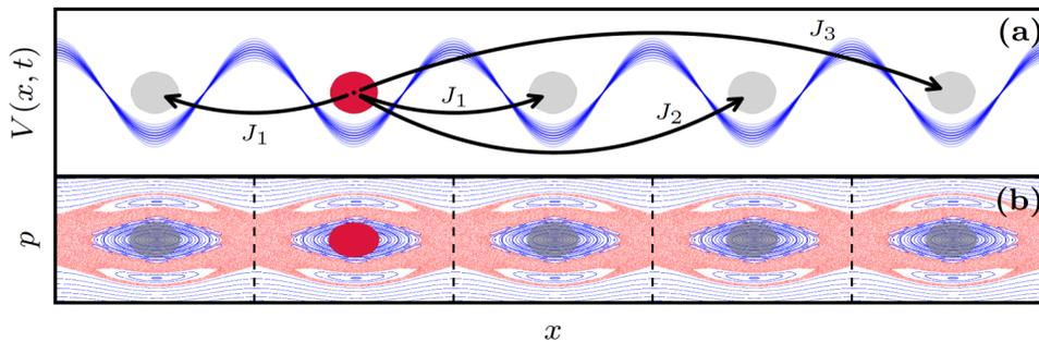
Figure 1: (a) Sketch of the system, showing the chaos-assisted hoppings  $J_n$  between regular islands, centered on the sites of the amplitude-modulated lattice (in blue), on which atoms are loaded. (b) Phase space (position  $x$ , momentum  $p$ ) representation. Regular islands (in blue) are embedded in the chaotic sea (in red).
