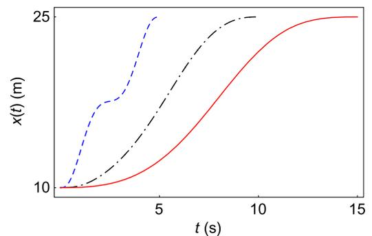
FIG. 2. Position of the trolley  $x(t)$  with respect to time for a dual operation with  $d = 15$  m,  $l_0 = 10$  m, and  $l_f = 5$  m.  $t_f = 15$  s, red solid line;  $t_f = 10$  s, black dashed-dotted line; and  $t_f = 5$  s, blue dashed line.
