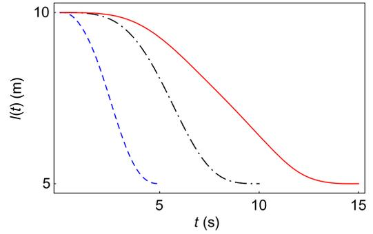
FIG. 1. Length of the rope with respect to time for a hoisting from  $l_0 = 10$  m to  $l_f = 5$  m.  $t_f = 15$  s, red solid line;  $t_f = 10$  s, black dashed-dotted line; and  $t_f = 5$  s, blue dashed line.
