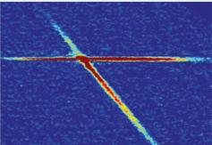
the atoms remains unchanged due to only weak coupling between the different modes in the crossing region. When the powers are roughly equal, the system enters the switching regime and the path of the atoms is completely switched to be guided by the crossing beam. Between these two regions exists the splitting regime, where all four beam paths become populated.
