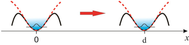
Figure 1. Schematic diagram of atomic transport in an effective one-dimensional Gaussian trap (dashed red line), approximated as a harmonic trap plus anharmonic quartic term (solid black line) from x = 0 to x = d .
