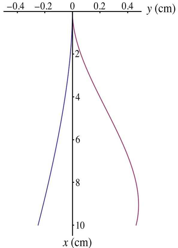
Fig. 4. Spring shape for the low-frequency resonance ( $\Omega = 60$  rad/s) on the left and the high-frequency resonance ( $\Omega' = 3800$  rad/s) on the right. The calculation is carried out using  $\chi = 2.1$ ,  $l = 10$  cm,  $h = 10$  cm, and  $\rho = 5$  cm.
