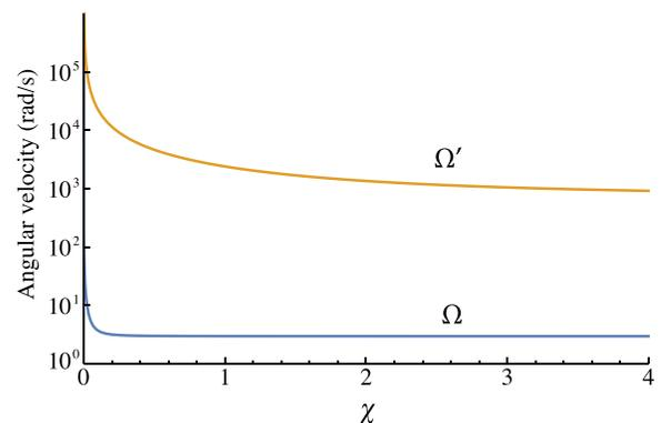
Fig. 3. The values of the low- and high-frequency roots  $\Omega$  and  $\Omega'$  of Eq. (22) are plotted as functions of  $\chi$  for a typical clock pendulum ( $h \approx 1$  m,  $\rho \approx 5$  cm, and  $l \approx 1$  cm). A typical  $\chi$  value for clocks is close to 2, for which  $\Omega$  is larger by only about 0.2% compared to if  $\chi$  were very large.
