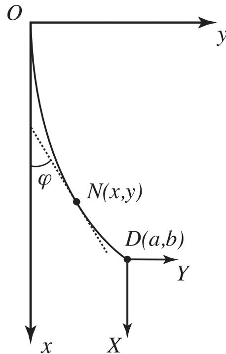
Fig. 2. Schematic of the spring that defines the notation used to analyze the spring shape. The point  $N$  (coordinates  $x, y$ ) lies on the spring and the tangent to the spring at  $N$  makes an angle  $\varphi$  with the  $x$ -axis. The spring is clamped in the pendulum rod at  $D$  (coordinates  $a, b$ ). The force exerted by the pendulum on the spring at  $D$  has components  $X$  and  $Y$ .
