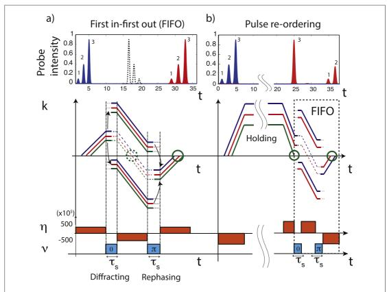
**Figure 3.** Re-ordering of pulses using two level atoms. From top to bottom: probe intensity as a function of time, evolution of the energy of the polariton in k-space and gradient slope and grating amplitudes used in the numerical simulations. (a) First in-first out scheme. (b) Pulse reordering.
