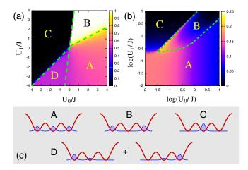
FIG. 2 (color online). (a)  $\langle \hat{n} \rangle / N$  as a function of  $U_{0,1}$  for N = 18. (b)  $\Delta \hat{\delta} / N$  in logarithmic scale for  $U_{0,1}$ . The dashed lines show the boundaries between the classical phases (A)–(D) that are shown schematically in (c).
