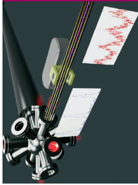
◀ Figure: Laser-cooled atomic packets are injected into a magnetic guide and slowed down by reflection on a moving magnetic barrier. The overlap of the successive slowed packets generates an ultraslow guided beam.
