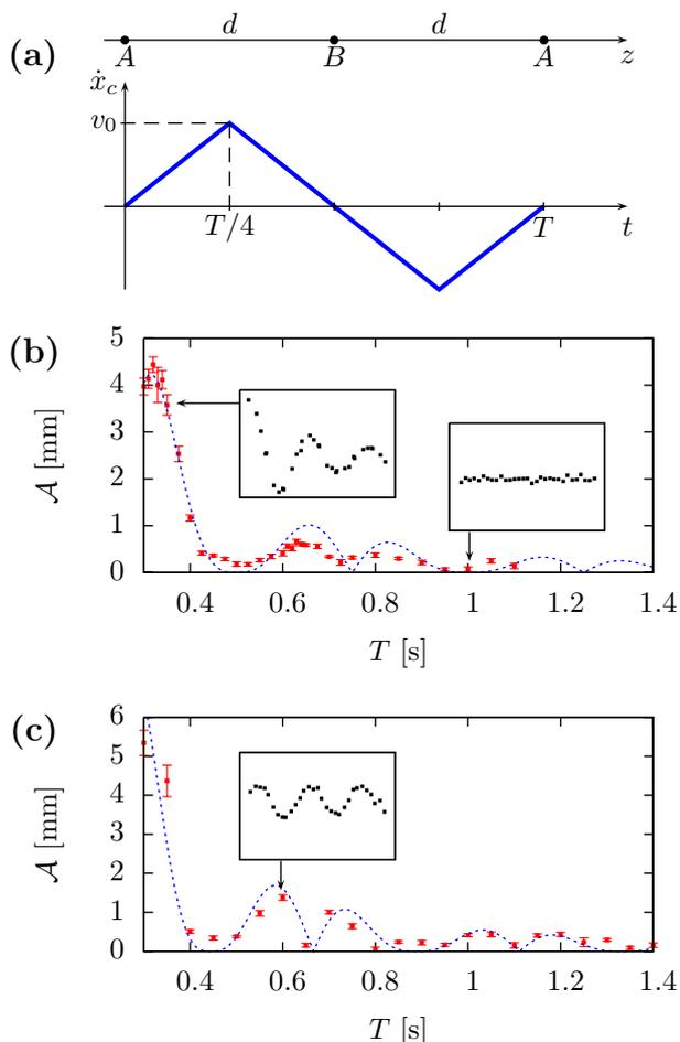
Fig. 2: (Colour on-line) (a) Velocity profile imposed to the trap to do the back and forth transport between  $A$  and  $B$  separated by  $d = 22.5$  mm. (b) (respectively, (c)) The measured amplitude  $\mathcal{A}$  of the centre-of-mass dipole oscillation for the conditions of scheme 1 (respectively, 2), see text. The dashed line is the theoretical prediction of eq. (4) with the measured angular frequency  $\omega_0$  of the trap.
